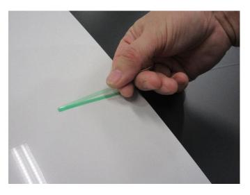
Press thumb firmly on folded edge, covering at least 1 cm tape. Firmly grasp the end of the tape with your thumb and index finger. Start with your two thumbs 1 cm apart. Bring thumbs together and give the tape a quick snap, breaking the carrier tape and exposing the filament (line).
