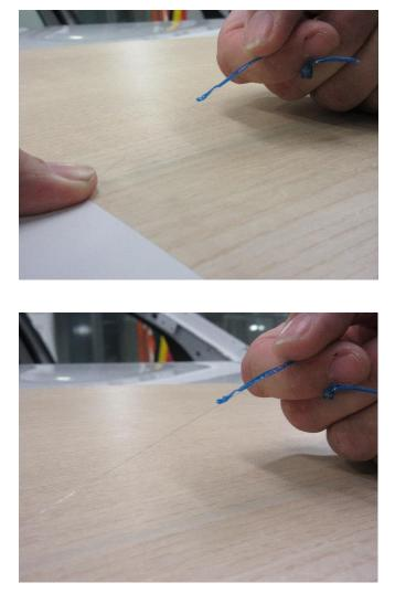
After cutting is finished, remove the excess film and the carrier tape from under the film. Assure that the carrier tape is completely removed without residuals.
