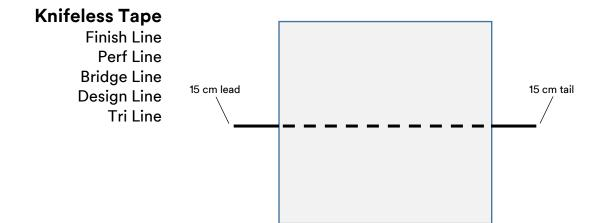
Begin with 15 cm of tape (before and after) where the graphic will be cut and lay down Knifeless Tape. Apply the film with pressure over the Knifeless Tape, leaving the lead and tail tape visible.
