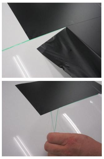
Heat the edges of the film and reapply the film edges with firm pressure.
