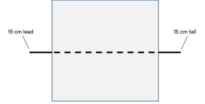
Begin with 15 cm of tape (before and after) where the graphic will be cut and lay down Knifeless Tape. Apply the film with pressure over the Knifeless Tape, leaving the lead and tail tape visible.
