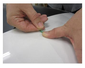
Pull the line back and not upward, stopping before the edge of the graphic.
