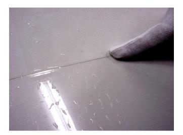
Take the cover tape and apply it over film and Knifeless Tape. Press the cover tape again firmly with your fingers.
