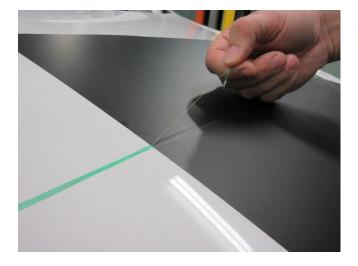
Fold the filament over the graphic. Press your thumb over both the filament and the graphic edge. Gently tug the filament to start cutting into the graphic, continuing to pull the line back and not upward.
