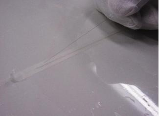
Tug the filament to start cutting into the film and the cover tape, continuing to pull the line back and not upward.
